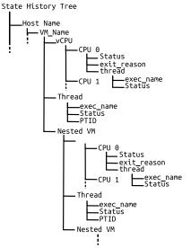
Fig. 5: State History Tree being used to store different information of VMs and nested VMs
